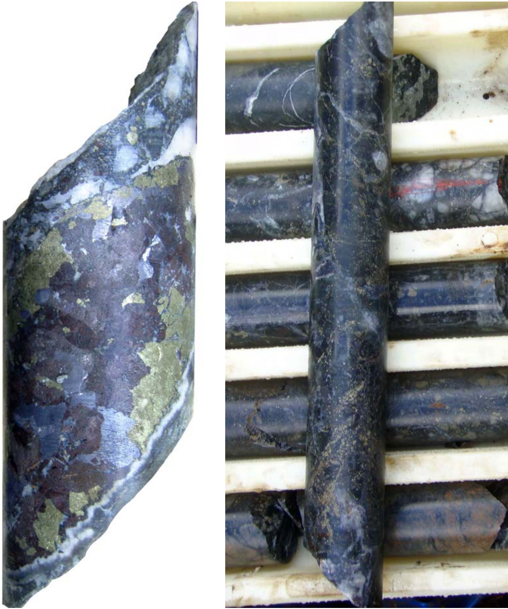
Figure 1. Photograph of 10cm wide vein containing abundant sphalerite, galena, pyrite and chalcopyrite (left) within sulphide-rich breccia zone (right) from DEVD2.
